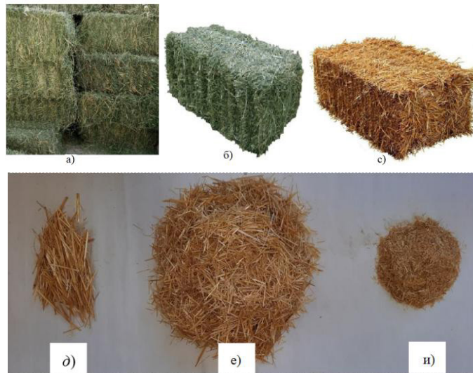
a) alfalfa presses; b) general view of alfalfa press; s) general appearance of pressed straw; d) fractions with a length greater than 50 mm, e) with a length of 30-50 mm and i) with a length of up to 30 mm
