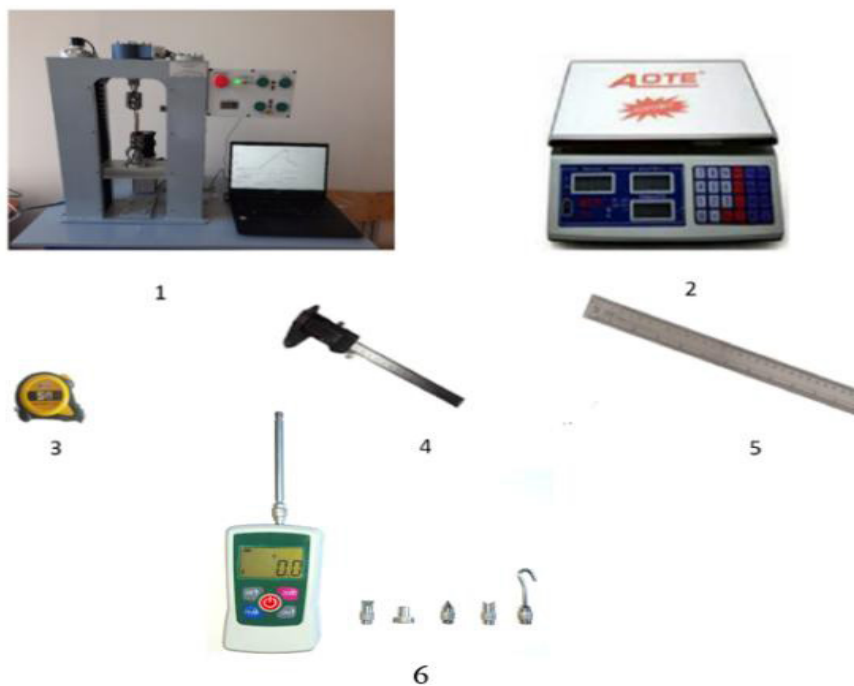
1 – UEIM-20-300 device; 2 – scales; 3 – roulette; 4 – barbell circle; 5 – ruler; 6 – DIGITAL FORCE GAUGE AMF-500 dynamometer.
