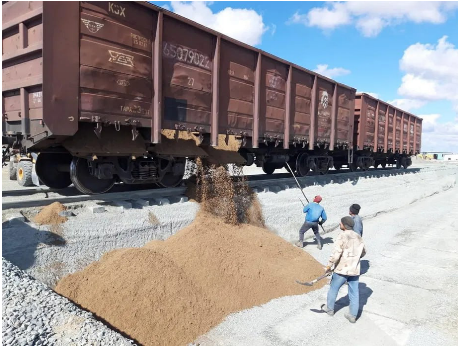
Figure 1. Fragments from the unloading process through the bottom hatches of a gondola wagon positioned on an elevated track
