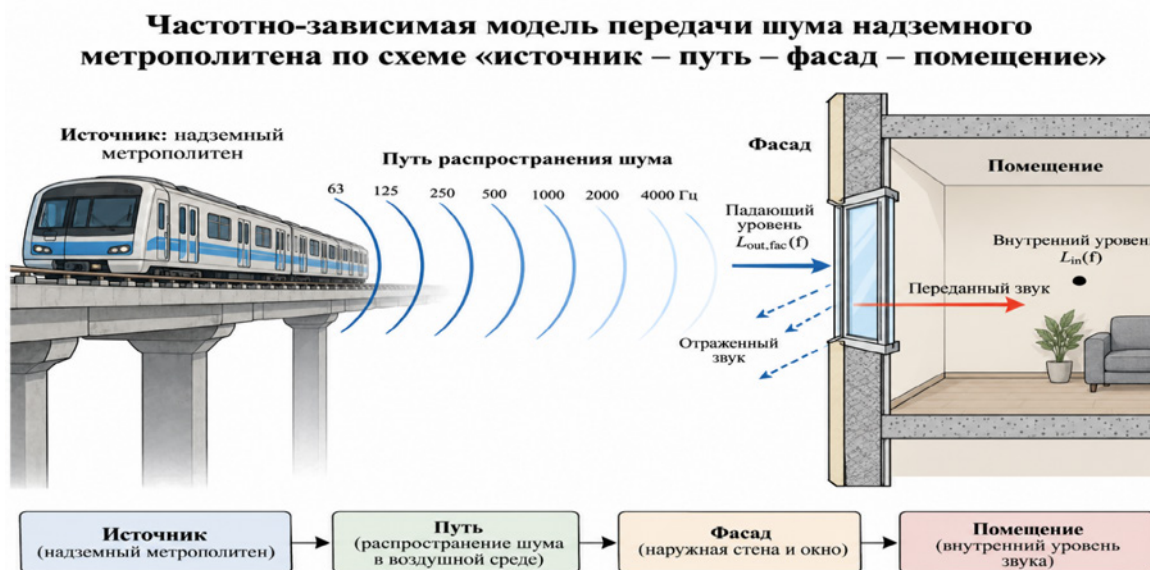
Figure 1. Frequency-Dependent Model of Noise Transmission from an Above-Ground Metro System Through the “Source–Propagation Path–Facade–Room” Framework 1
